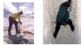
Ablation stake, snow pit measurement (Photos by D. Vonder Muehl, M. Hoelzle)
