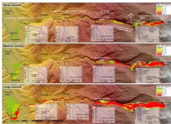
Model simulations of ice avalanche, impact waves and lake outburst flood for Laguna 513 / Carhuaz, Peru (Schneider et al. 2014). This information was used to generate hazard maps for the area.
