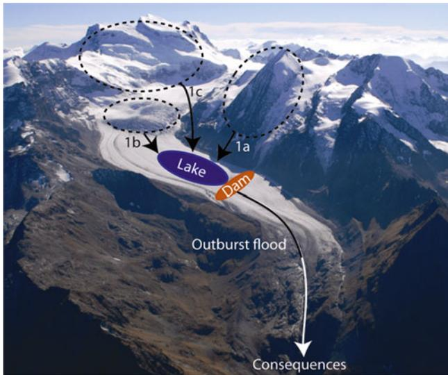
**Fig. 1** Scheme of the investigated process chain, illustrated with the example of the potential future lake Corbassière, Switzerland. *Dashed lines* = possible detachment zones of rock- (*1a*), ice- (*1b*) or combined rock/ice-avalanches (*1c*). Picture: U. Bläsi ([www.airbox.ch/air/](http://www.airbox.ch/air/))
